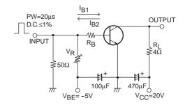
$20I_{B1} = -20I_{B2} = I_C = 5A$ For PNP, the polarity is reversed.
